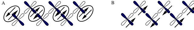
Fig. 3 – A sketch of the zero-temperature states. The lobes of the orbitals that lie in the plane of the titanium chain are depicted. The dark lobes are occupied orbitals. (A) Orbital-assisted Peierls state with spin valence bonds. (B) Alternating ferro and antiferro spin bonds as found in the classical spin model and density functional studies.
