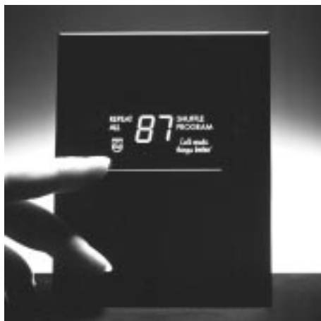
Figure 1.1: A polymer LED display. (Source: “Philips Components to set up light-emitting polymer business”, Philips Research Press release 9802e/March 1998)
