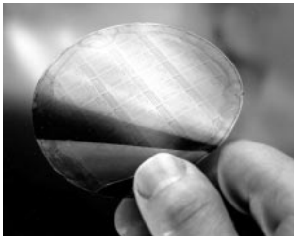
Figure 1.6: Integrated circuits built out of all-polymer transistors still operate when the foils are sharply bent, making them ideally suited for integration as electronic identification tag or antitheft sticker into product wrappings for soft packages. (Source: “New plastic circuits are flexible enough to be folded in half”, Philips Research Press release 97005e/ 8 December 1997)
