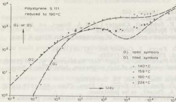
Fig. 17.  $G'_R$  and  $G''_R$  calculated from Eqs (II. 47) - (II. 50), with  $M_e = 30,000$ .
