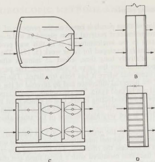
Fig. 5 Four types of image intensifier, A. Electronoptical image intensifier. B. Solid state image intensifier. C. Secondary emission image intensifier. D. Channelled image intensifier.
