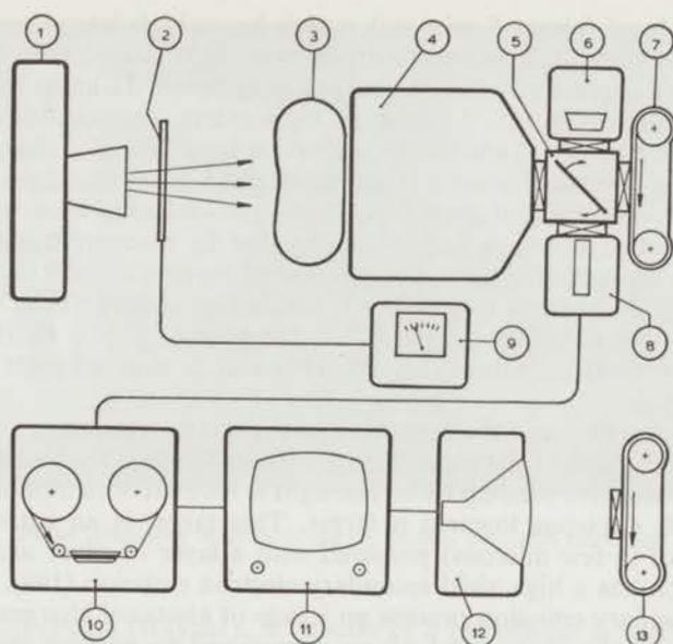
Fig. 6. General diagram of television fluoroscopy. 1. x-ray tube. 2. flat ionization chamber. 3. patient. 4. image intensifier. 5. image divider. 6. photographic camera. 7. film camera. 8. television camera. 9. measurement of incident radiation energy. 10. video recorder. 11. television monitor. 12. kinescope. 13. film camera.
