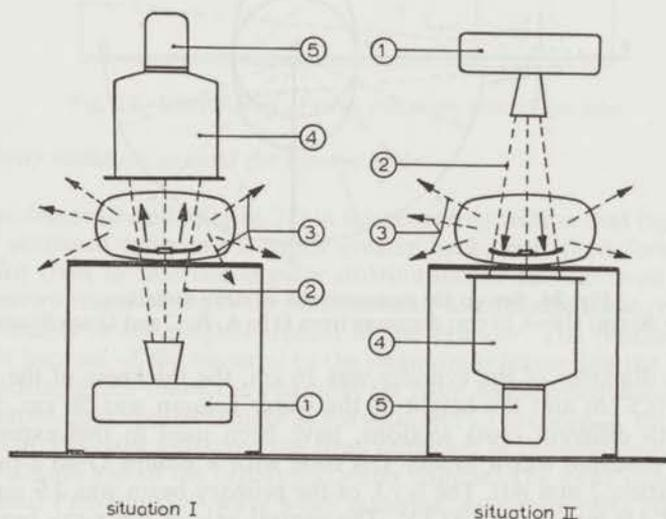
Fig. 23. Two situations for television fluoroscopy.
