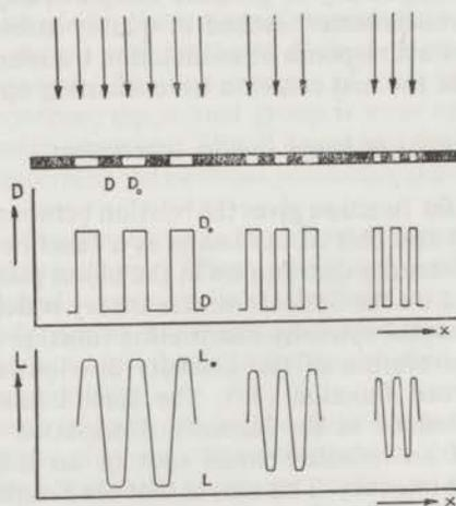
Fig. 2. Determination of modulation transfer of spatial frequencies.
