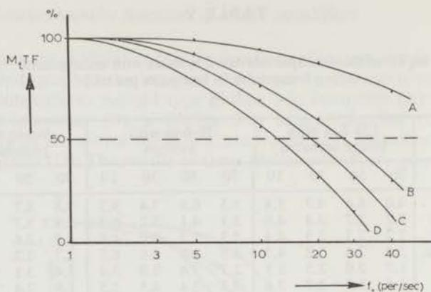
Fig. 15. Modulation transfer functions of time frequencies.
