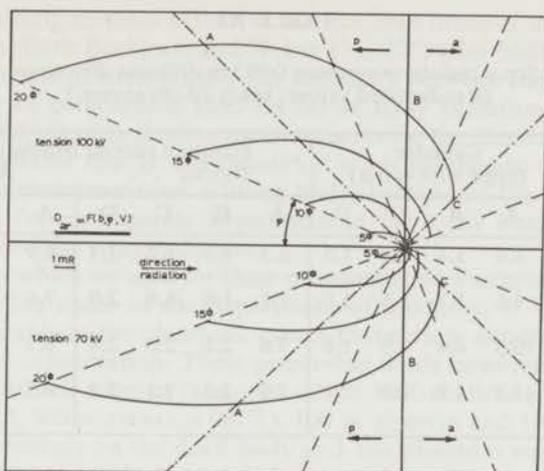
Fig. 25. Distribution of stray radiation around cylinder.
