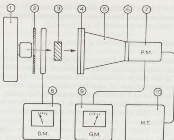
Fig. 9. Measurement of the conversion function.
