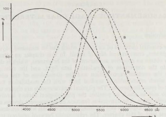
Fig. 8. Relative spectral sensitivities of the eye (CIE) and of the detector A. scotopic vision B. photopic vision C. photomultiplier D. photomultiplier with correction filters
