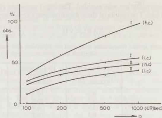
Fig. 19. Observability measured on two fluoroscopic screens. Screen I: Helia; Screen II: Levy West III; h.c. = high contrast; l.c. = low contrast
