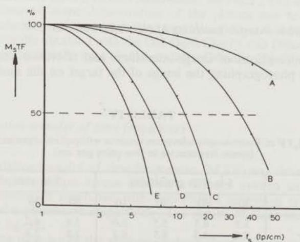
Fig. 13.  $M_s$ TF for different photographic methods.
