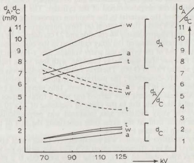
Fig. 26. Stray radiation around the phantom and the water volume
