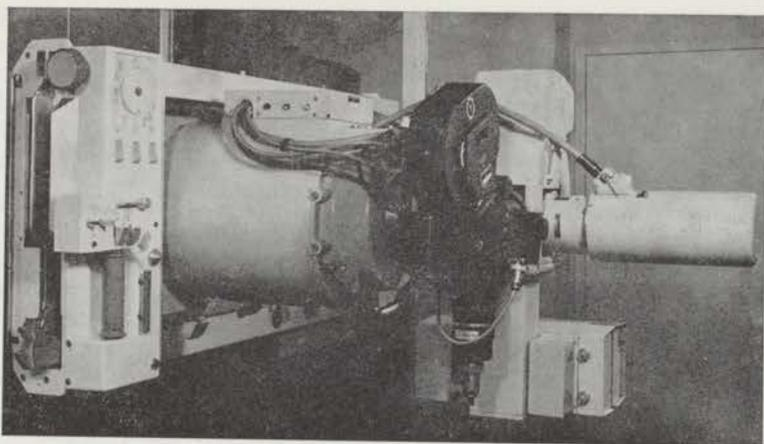
Fig. 8. Image intensifier with cameras for photo, cine and television pick-up.
