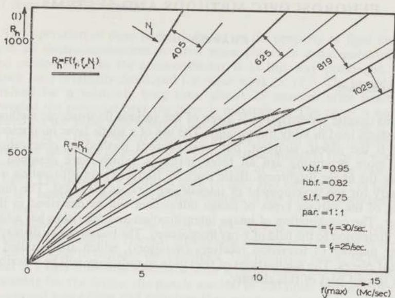
Fig. 4 Relations between resolution and bandwidth
