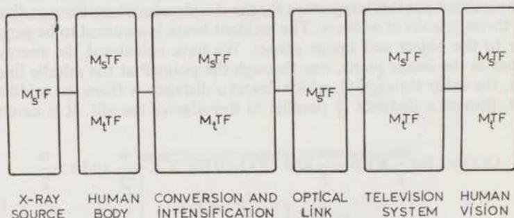
Fig. 3. Image deterioration in fluoroscopy.
